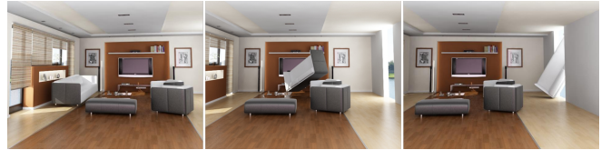
Fig. 1. Living Room Benchmark: This figure shows three image shots of getting the sofa out through a door, which creates narrow passages in 6 dof configuration space. Our method achieves ten and two times improvements over a basic RRT and an optimization-based retraction method respectively.
