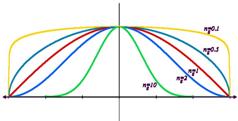
How the shape of the highlight changes with varying n<sub>s</sub>
