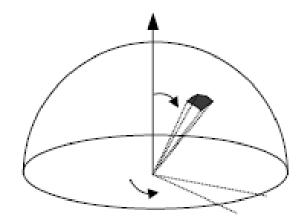
$$\langle I \rangle = \frac{1}{N} \sum_{i=1}^{N} \frac{f(\varphi_i, \theta_i) \sin \theta}{p(\varphi_i, \theta_i)}$$
