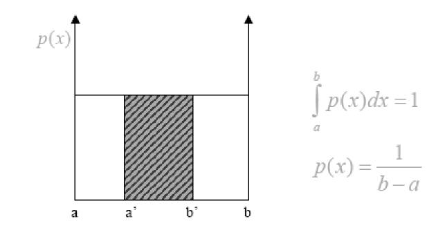
Probability that x belongs to  $[a',b'] = \int_{a'}^{b'} \frac{1}{(b-a)} dx = \frac{(b'-a')}{(b-a)}$  $\Pr(x \le y) = CDF(y) = \int_{-\infty}^{y} p(x) dx = \frac{(y-a)}{(b-a)}$
