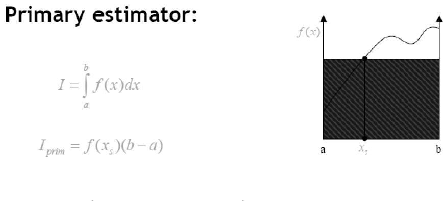
$$E(I_{prim}) = \int_{a}^{b} f(x)(b-a)p(x)dx = \int_{a}^{b} f(x)(b-a)\frac{1}{(b-a)}dx = I$$
