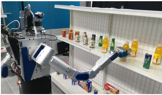
Fig. 6. This figure shows our experimental environment mimicking a convenient store with the mobile Hubo robot. There are various kinds of beverages and snacks on the shelf, and our goal is to grasp the yellow beverage. Our approach computes a shorter path over the decoupled approach in the same time budget.
