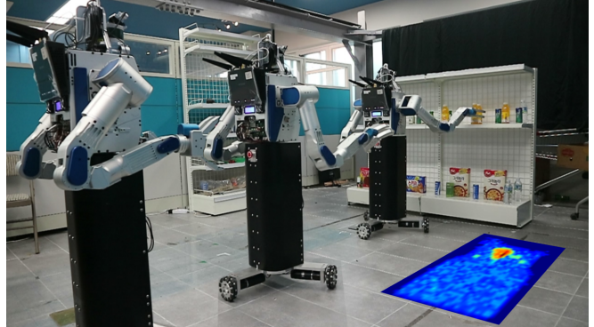
Fig. 1. This figure shows a sequence of the mobile Hubo robot grasping the yellow beverage. The heat map on the bottom right represents a sample density in terms of the 2D floor projected from samples generated from our harmonious sampling in the joint C-space consisting of the base and the manipulator. Samples are distributed intensively near the goal configuration, resulting in efficient and effective exploration of solution paths.
