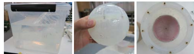
Water-resistant test (passed 12h submersion test)
