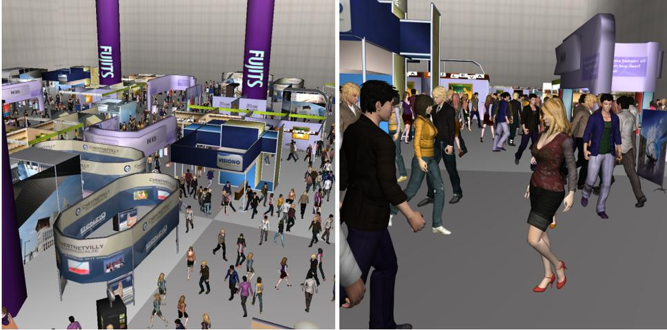
Figure 3.1: [ This figure shows two images of an exhibition crowd scene that has 1 K articulated characters. All the characters and the scene have 83 M triangles. Our method achieves 46 frames per second (fps) on average for this model with 0.5 pixel-of-error (PoE) in a 1280 by 720 HD screen resolution. ]
