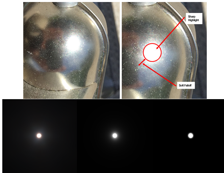
Figure 17.4: The top image row shows a captured image of a metal and its main characteristics, the strong highlight in the center and a smooth falloff. These images are created by Neil Blevins. In the bottom row, from the left, the captured image (highlight) of a chrome, rendered images by GGX, and Beckmann distributions. The GGX has a long tail and thus represents the soft falloff of the highlight. These images are excerpted from [Bur12].
