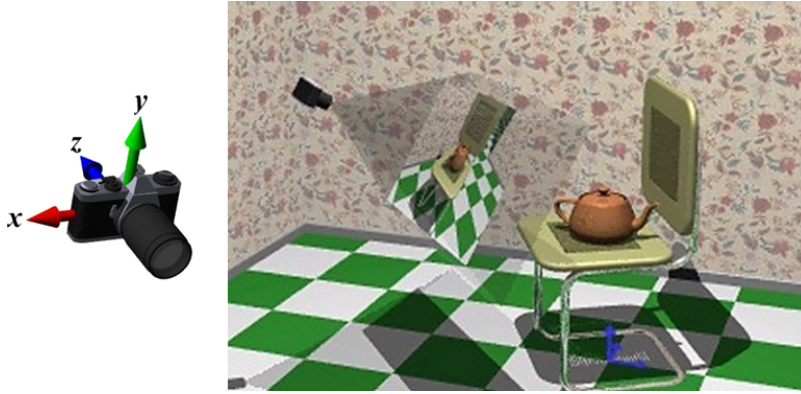
Figure 4.1: To generate an image, we specify a camera in the world space, which consists of the origin and X, Y, and Z axis of the camera.
